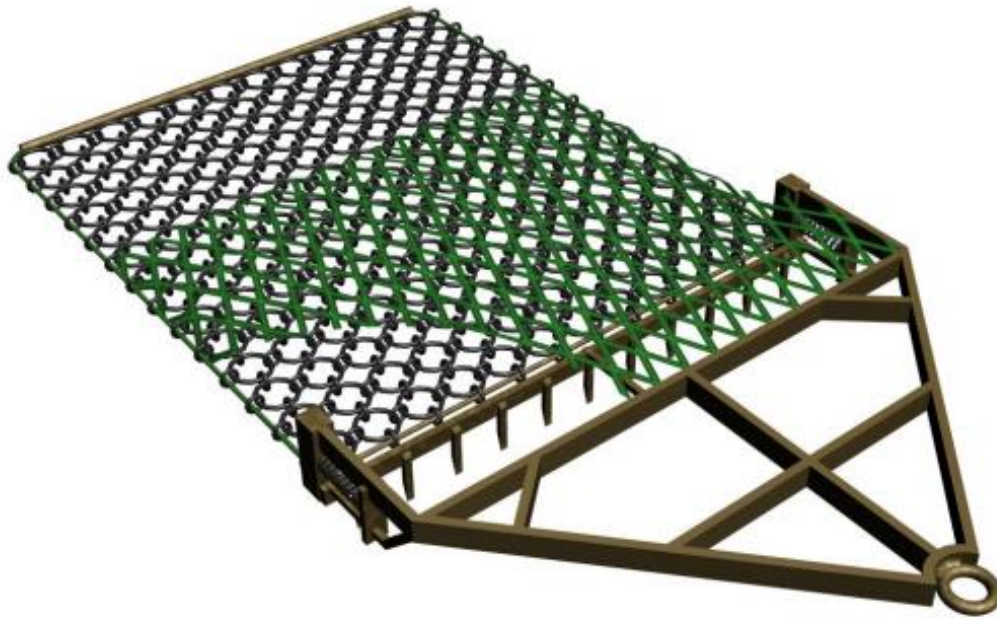
Figure 5: A diagram representing a Newhaven scallop dredge
